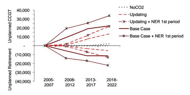
Figure 7 Cumulative installed capacity in CCGT and retired capacity, double CO<sub>2</sub> price
