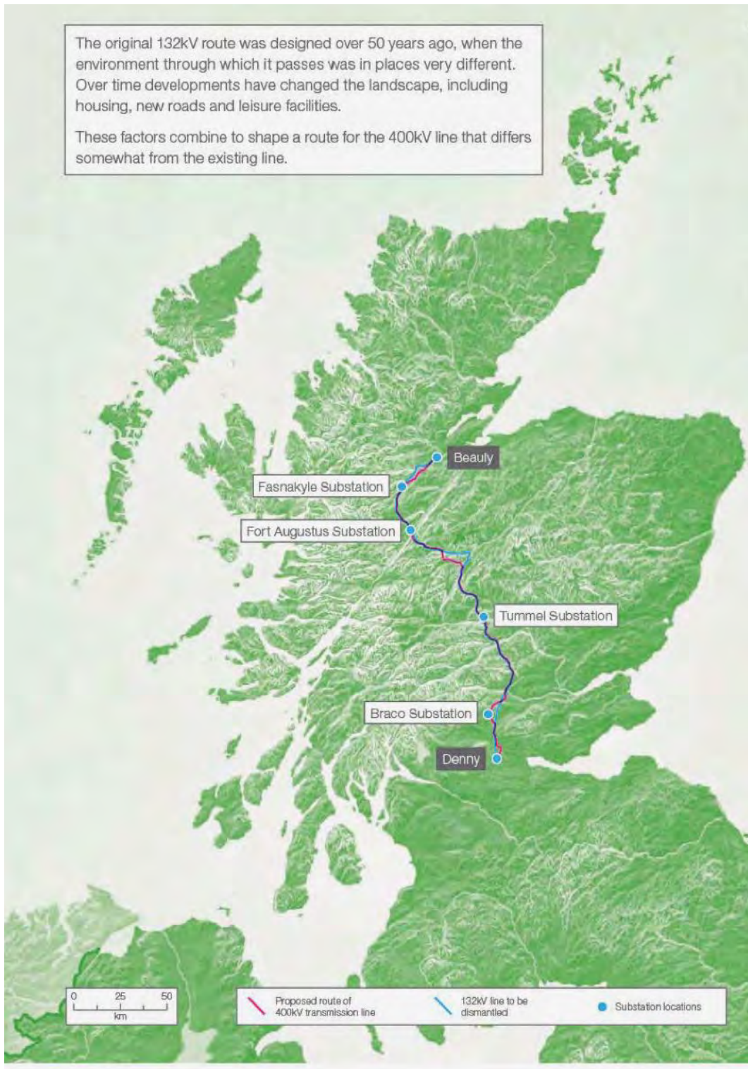
Figure 3.1, Overview of the Beaully-Denny power-line routing.
