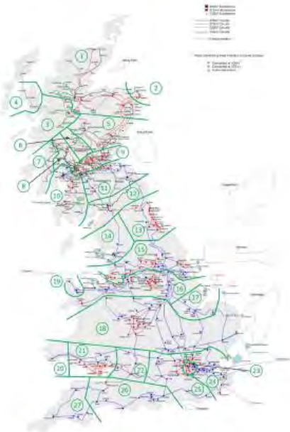
Figure A2: GB Existing Transmission System
