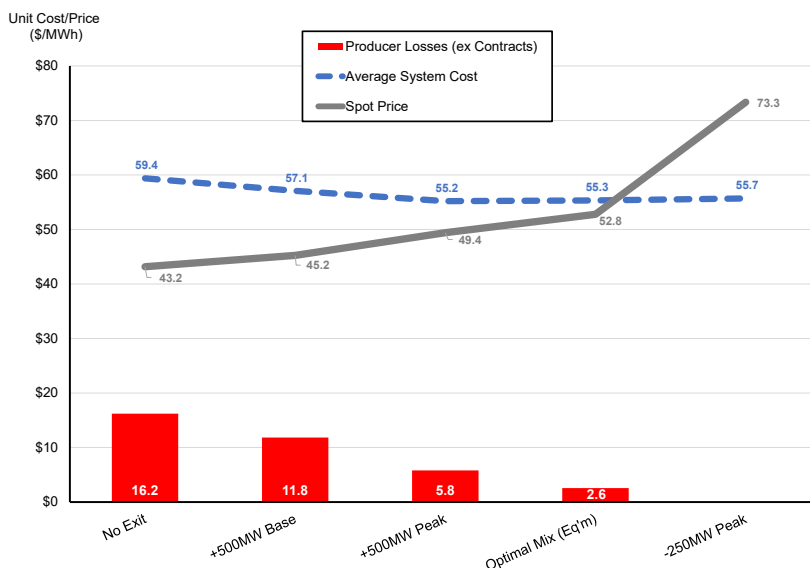
Figure 15: Scenario 4 (35% VRE) plant stock sensitivities +/- base and peaking plant
