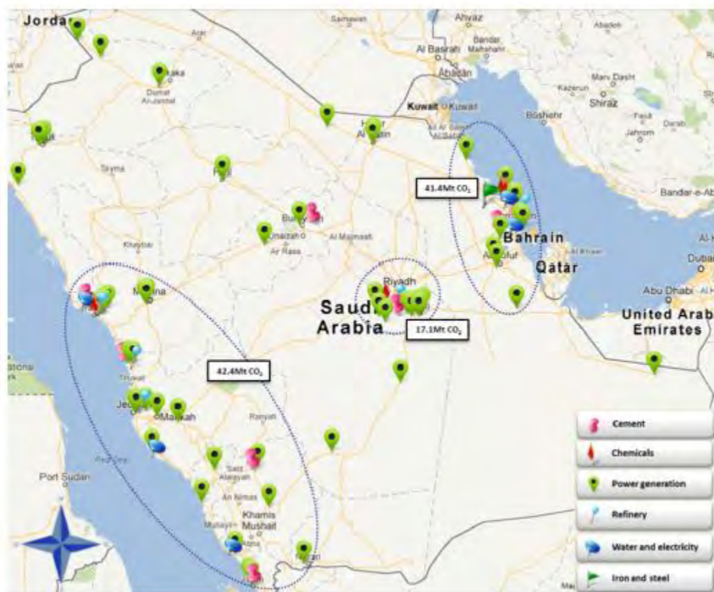
Figure9: Large stationary emissions sources by type in Saudi Arabia. (Source: Liu et al., The role of CO2 capture and storage in Saudi Arabia's energy future. International Journal of Greenhouse Gas Control , 2012; dx.doi.org/10.1016/j.ijggc.2012.08.008 )
