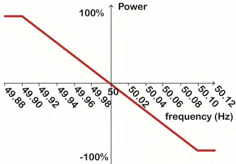
Fig. 3: Droop control signal for FCR-N in the Nordics
