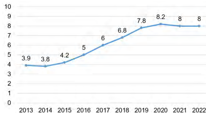
Fig 1. Average power rating of installed turbines in Europe, 2013-22 [ Error! Reference source not found. ] (MW).
