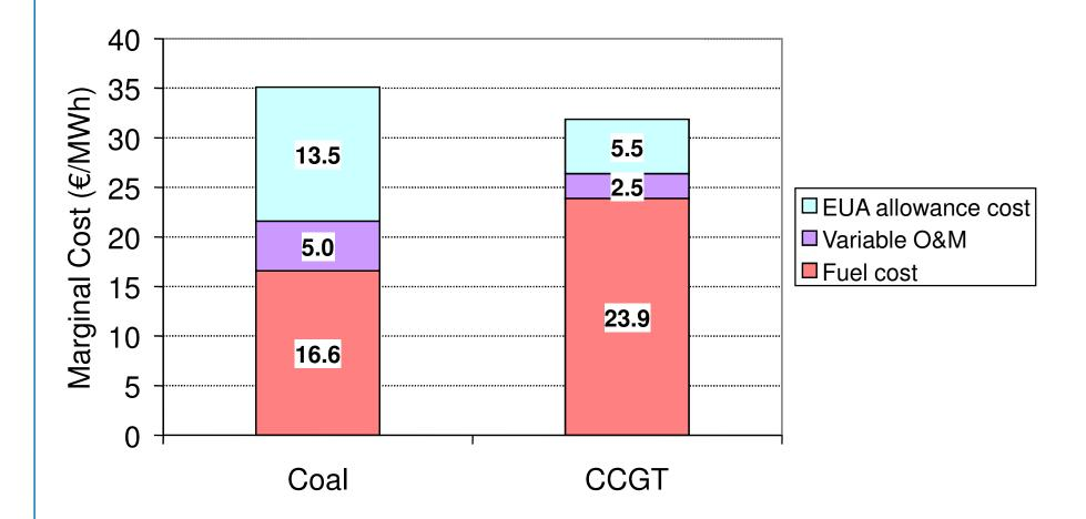
Note: Based on efficiency ratings of 36% and 50% net HHV efficiency respectively. €15/tCO2. Price of gas at 3.50€/MMBTu (35€c/therm) and coal at 1.75 €/MMBTu (42€/tonne at 6,000kcal/kg).
