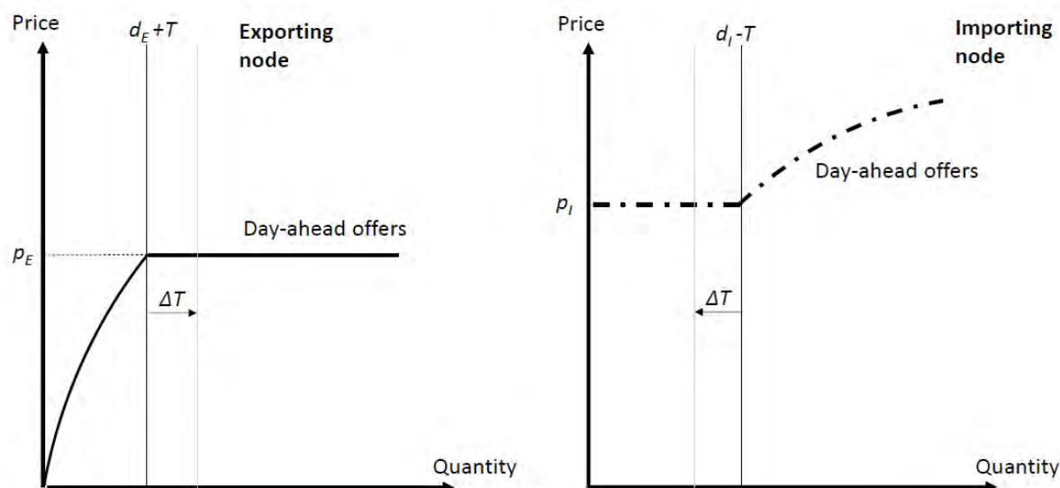
Figure 3: The equilibrium in a day-ahead market with two nodes/zones, where the cross-zonal transmission capacity between the two nodes has been exaggerated by \Delta T .
